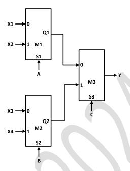
For an instance of inputs X1=1, X2=1, X3=0, and X4=0, the number of combinations of A, B, C that give the output Y=1 is \_\_\_\_\_
